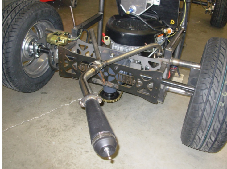
Exhaust system fully installed (Above).
